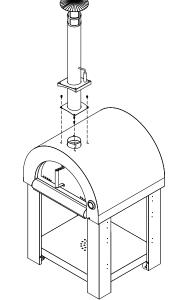
6/. Installed chimney cap with 4pcs of 5/32"\*10mm screws
