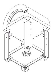
3/. Ash support installment with 4pcs of 1/4"\*15mm screws
